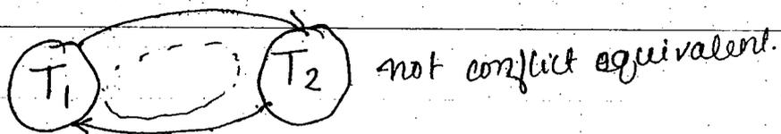
b)  $R_1(X), R_2(Y), W_3(X), R_2(X), R_2(Y), C_1, C_2$
