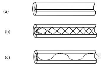
Figure 2.2.5 Schematics of three optical fiber types, (a) Single-mode step-index, (b) Multi-mode step-index, and (c) Multi-mode graded-index
