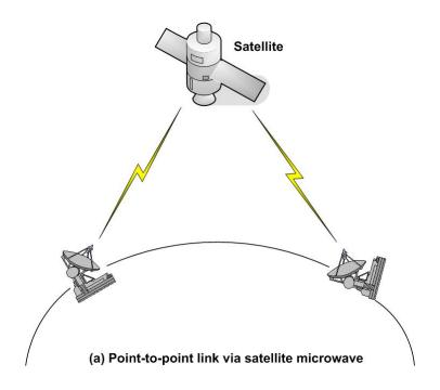
Figure 2.2.7 Satellite Microwave Communication: point -to- point
