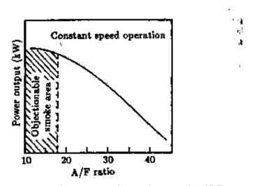
Fig. 10.16 Effect of A/F Ratio on Power Output of a CI Engin
