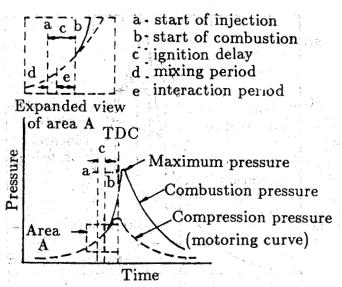
Fig1.Stages of combustion
