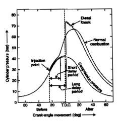
availability for simultaneous explosion, is too great, which results in rapid pressure rise. The delay period should be as short as possible since long delay period gives more rapid rise in pressure and thus causes knocking.
