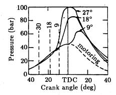
Effect of Injection Timing on Indicator Diagram
