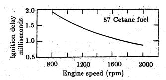
in degrees of crank travel the delay period increases as the engine operates at a higher rpm. The fuel pump is geared to the engine, and hence the amount of fuel injected during the delay period depends on crank degrees and not on absolute time. Hence, at high speeds, there will be more fuel present in the cylinder to take part in the second stage of uncontrolled combustion resulting in high rate of pressure rise.
