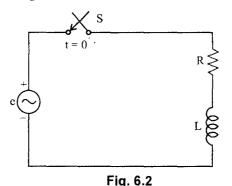
Let  $e = E_{max}$  Sin ( $\omega t + \alpha$ ) when the switch S is closed at  $t = 0^+$  $e = E_{max}$  Sin ( $\omega t + \alpha$ ) = R + L  $\frac{di}{dt}$
