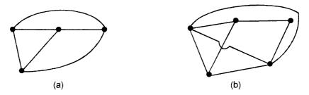
Fig. 2.1 (a) Planar Graph (b) Non-Planar Graph.
