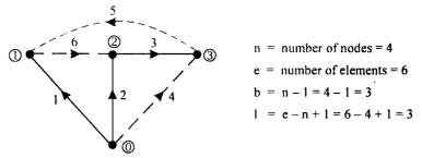
Fig. 2.4 (a) Tree for the system in Fig. 2.3.
