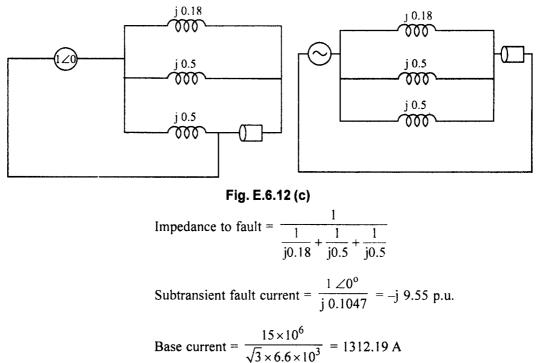
Subtransient fault current =  $1312.19 \times (-j 9.55)$
