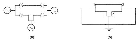
Fig. 2.2 (a) Power system single-line diagram (b) Positive sequence network diagram
