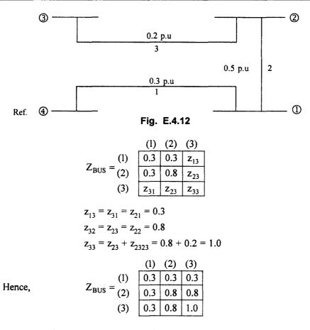
Step-4 Add element (4) which is a link a = 4; b=3. The augmented impedance matrix with the fictitious node 1 will be.
