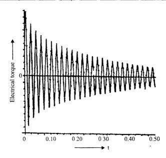
Fig. 6.5 Electrical torque on three-phase terminal short circuit.
