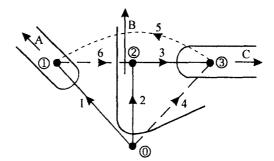
Fig. 2.7 Cut-set for the tree in Fig. 2.4(a).
