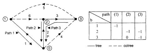
Fig. 3.4 Branch-Path Incidence Matrix for network
