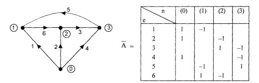
Fig. 3.1 Element-node incidence-matrix for the graph of Fig. (2.3).
