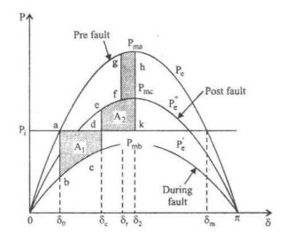
Fig. 8.15 Fault clearance and reclosing.
