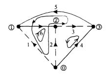
Fig. 2.4 (b) Co-tree for the system in Fig. 2.3.
