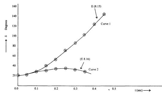
E8.16 If the fault in the previous example E.8.14 is cleared at the end of 2.5 cycles determine the swing curve and examine the stability of the system.
