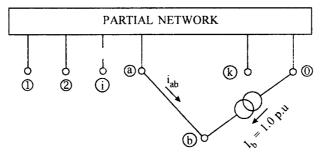
Fig. 4.6 Partial Network with Branch Added (Calculations of Self Impedance).
