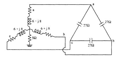
Converting the delta connected capacitor tank into star
