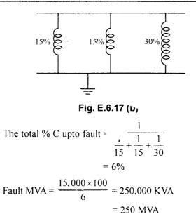
(ii) If the fault occurs at  $F_2$ , the reactance diagram will be as in Fig. E.6.17 (c).
