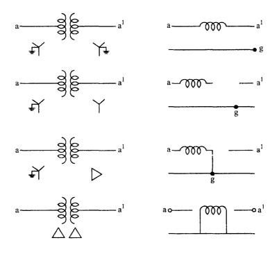
Fig. 7.5 Zero sequence equivalent circuits.
