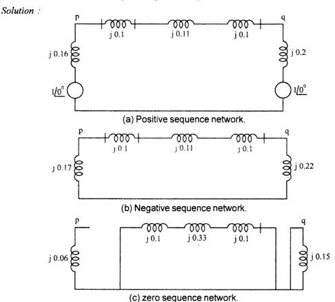
The three sequence networks are shown in Fig. (a,b and c). For a line-to-ground fault an phase a, the sequence networks are connected as in Fig. E. 7.9 (d) at bus 'q'.
