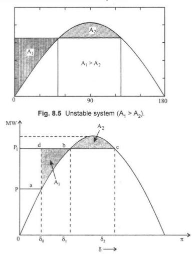
Fig. 8.6 Transient stability limit.
