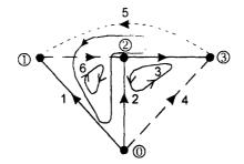
Fig. 2.5 Basic loops for the tree in Fig. 2.4(a).
