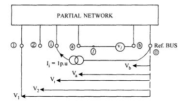
Fig. 4.7 Addition of a Link (Calculation of Mutual Impedance).
