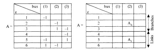
Fig. 3.3 Partitioning of matrix A.
