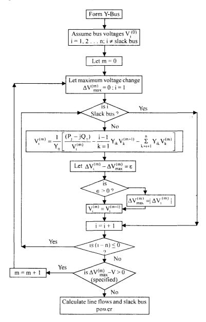
Fig. 5.3 Flowchart for Gauss – Seidel iterative method for load flow solution using Y-Bus.
