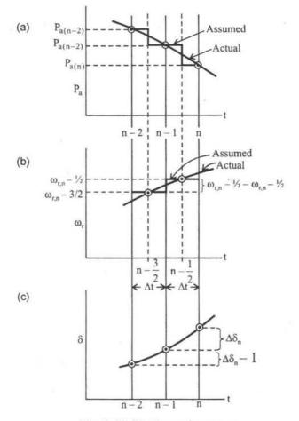
Fig. 8.16 Plotting swing curve.
