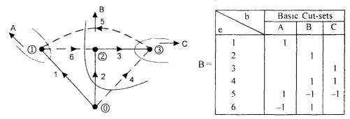
Fig. 3.5 Basic Cut-set incidence matrix for the graph in 3.5(a) drawn and shown.
