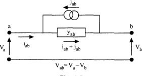
y<sub>ab</sub> is the self admittance of the network element a-b
