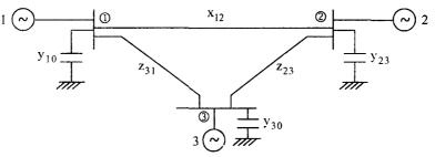
Fig. 5.2 Three bus transmission system.
