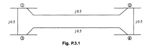
P 3.2 Compute the bus admittance matrix for the power shown in figure by (i) direct inspection method and (ii) by using singular transformation.
