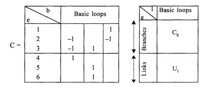
Fig. 3.9 Partitioning of basic loop incidence matrix.
