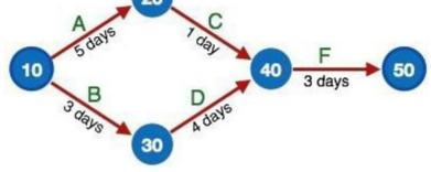
Events are shown as numbered nodes. They are connected by labeled arrows depicting the sequence of tasks in the project.
