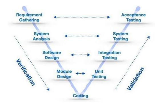
At every stage, test plans and test cases are created to verify and validate the product according to the requirement of that stage. For example, in requirement gathering stage the test team prepares all the test cases in correspondence to the requirements. Later, when the product is developed and is ready for testing, test cases of this stage verify the software against its validity towards requirements at this stage.
