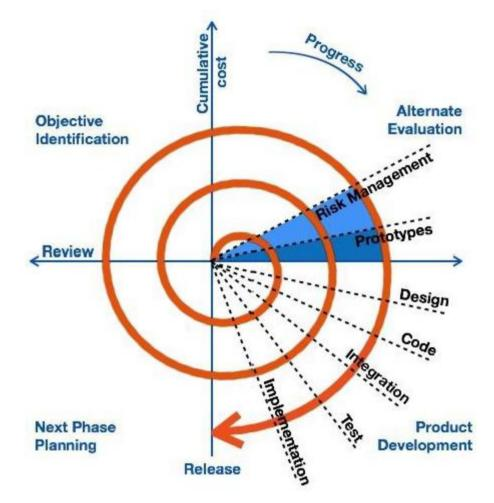
This model considers risk, which often goes un-noticed by most other models. The model starts with determining objectives and constraints of the software at the start of one iteration. Next phase is of prototyping the software. This includes risk analysis. Then one standard SDLC model is used to build the software. In the fourth phase of the plan of next iteration is prepared.
