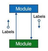
• **Control flow** - A directed arrow with filled circle at the end represents control flow.
