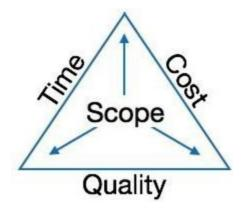
The image above shows triple constraints for software projects. It is an essential part of software organization to deliver quality product, keeping the cost within client's budget constrain and deliver the project as per scheduled. There are several factors, both internal and external, which may impact this triple constrain triangle. Any of the three factors can severely impact the other two.
