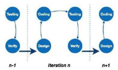
The software is first developed on very small scale and all the steps are followed which are taken into consideration. Then, on every next iteration, more features and modules are designed, coded, tested, and added to the software. Every cycle produces a software, which is complete in itself and has more features and capabilities than that of the previous one.
