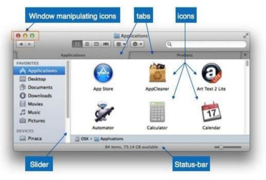
**Window** - An area where contents of application are displayed. Contents in a window can be displayed in the form of icons or lists, if the window represents file structure. It is easier for a user to navigate in the file system in an exploring window. Windows can be minimized, resized or maximized to the size of screen. They can be moved anywhere on the screen. A window may contain another window of the same application, called child window.
