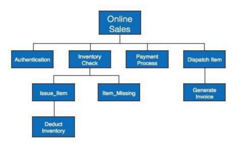
In contrast to Input Process Output (IPO) diagram, which depicts the flow of control and data in a module, HIPO does not provide any information about data flow or control flow.
