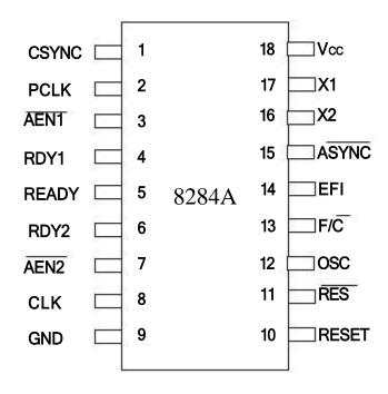
Fig1. Pin diagram of the 8284A clock generator
