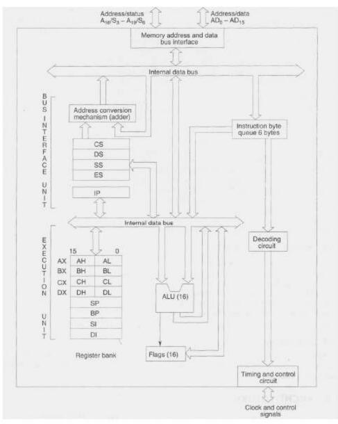
Fig1.2. Internal architecture of 8086 Microprocessor
