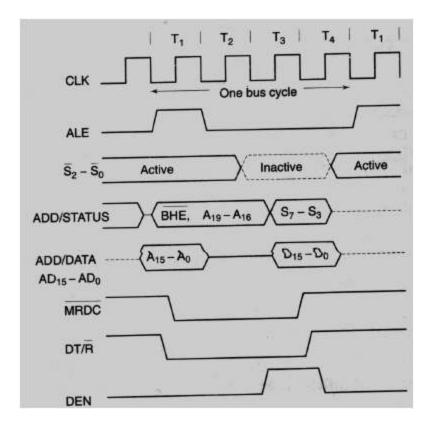
Fig. 1.2 Memory Read Timing in Maximum Mode
