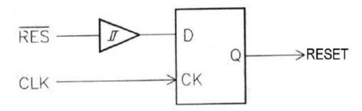
The Reset logic generates the Reset input signal for the 8086/8088. When the RESET\* pin goes low, the Reset output is generated by the 8284 when the next clock transition takes place.
