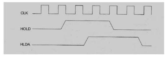
Fig 1.4. Bus Request and Bus Grant Timings in Minimum Mode System
