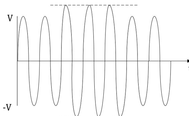
Figure 2.3 Voltage Swell typical waveform
