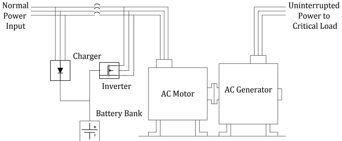
Figure 2. 9 Rotary uninterruptible power source (RUPS) system using a battery bank
