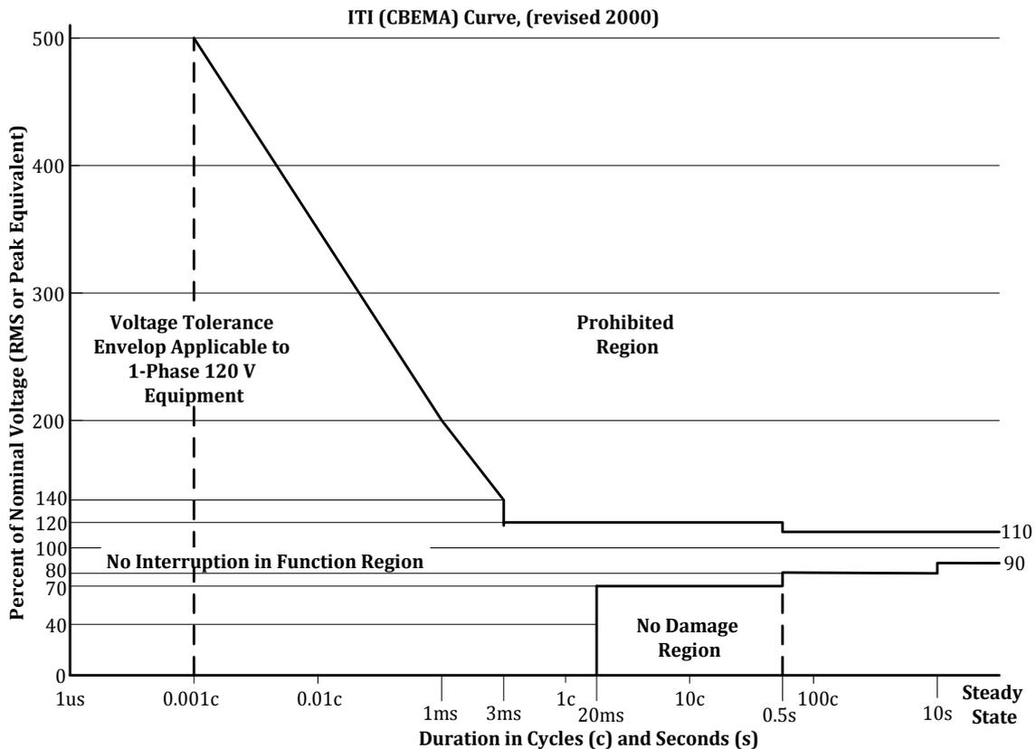
Figure 2. 10 Information Technology Industry Council (ITIC) graph providing guidelines as to the voltage tolerance limits within which information technology equipment should function satisfactorily. (Courtesy of the Information Technology Industry Council, Washington, D.C.)
