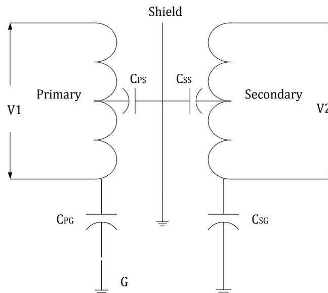
Figure 2.4 Common mode noise attenuation by shielded isolation transformer
