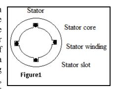
stator flux is running with synchronous speed ( $N_s = \frac{120 \text{ f}}{P}$ ) along with stator core.
