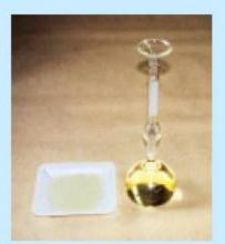
Le Chatelier flask - ASTM C 188 Standard Test Method for Density of Hydraulic Cement
