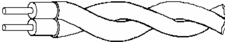
**Figure 2.2.2** CAT5 cable (twisted cable)
