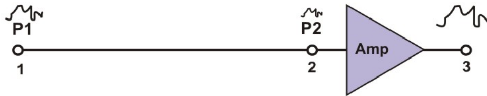
Figure 2.3.1 Compensation of attenuation using an amplifier
