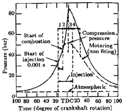
*Fig 1. Stages of combustion*
