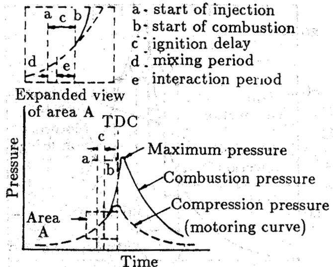
*Fig 2. Pressure Time diagram illustrating Ignition delay*
