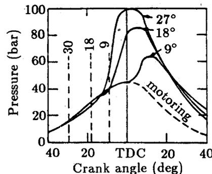
Effect of Injection Timing on Indicator Diagram
