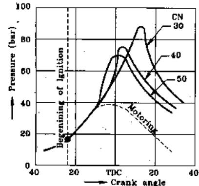
Fig. 18.2. Effect of CN on indicator diagram.
