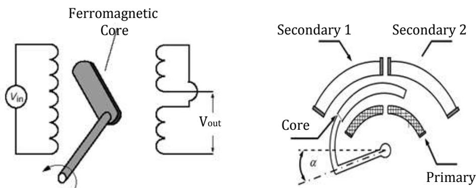
Figure 5.3 Diagram of Rotary Variable Differential Transformer (RVDT)
