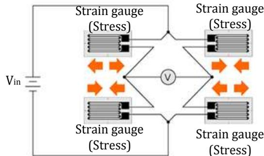
Figure 5. 4 Diagram of full-bridge strain gauge
