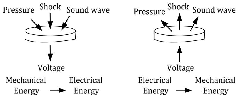
Figure 5. 5 Diagram of piezoelectric transducer
