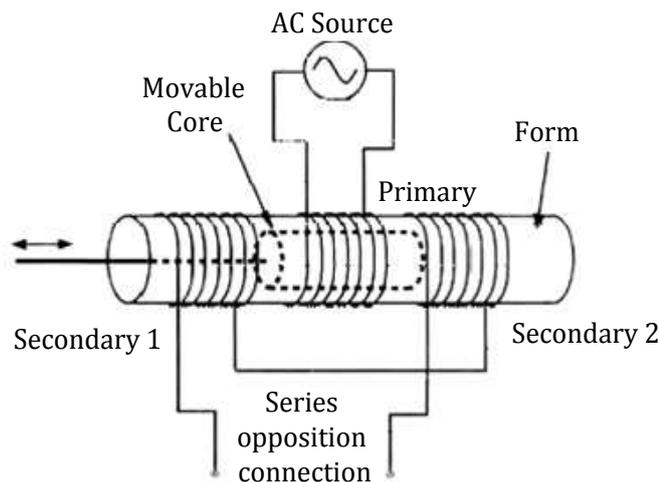
Figure 5.2 Diagram of Linear Variable Differential Transformer (LVDT)
