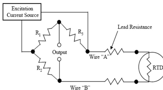
Figure 5. 6 Circuit diagram of two wire RTD bridge circuit
