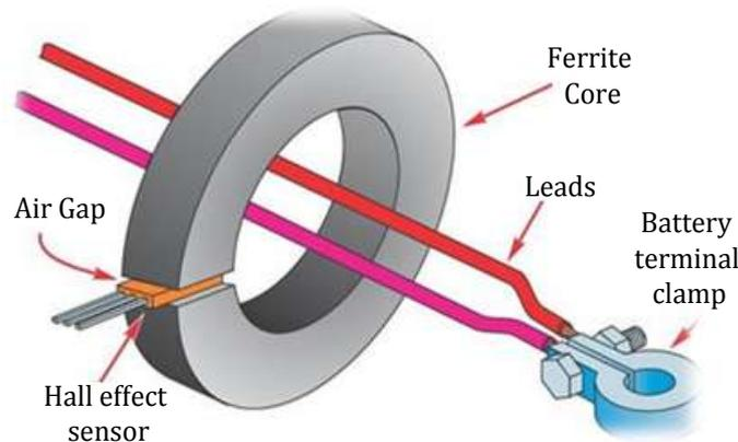
Figure 5. 8 Typical arrangement of Hall Effect sensor
