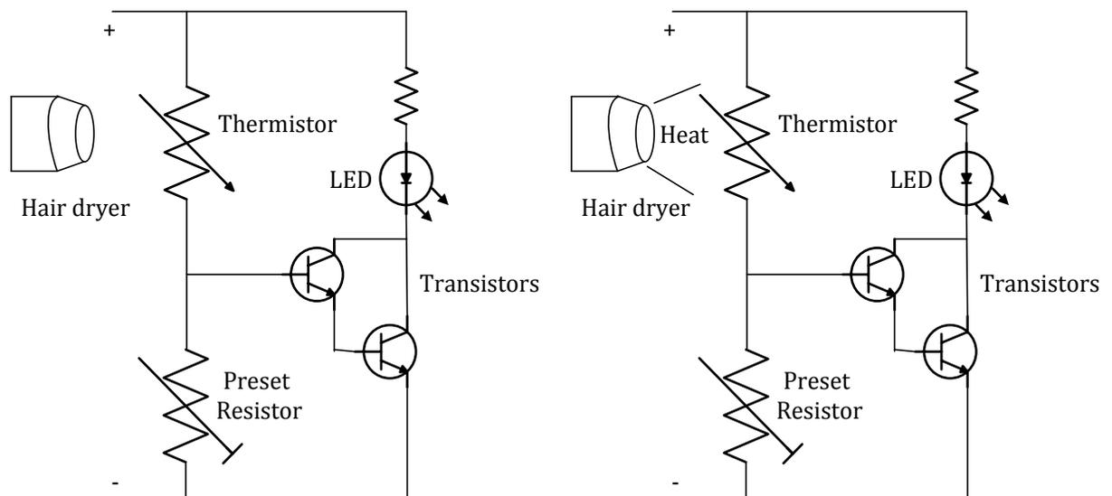
Figure 5. 7 Application circuit of Thermistor
