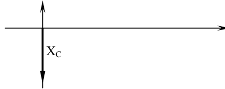
Figure 12-20 Impedance diagram of a capacitor.
